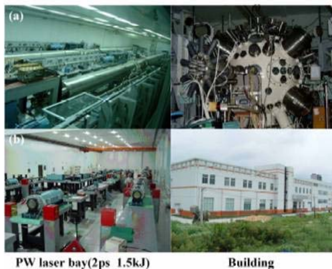
Fig. 1. (a) SG-II laser bay and target chamber, (b) the ninth laser beam to be PW laser.
